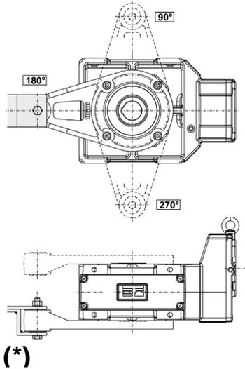
Fig. 17: Helical bevel gear unit
