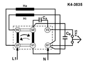
Figure 14. Single phase motor type SE(M)(K, L)h-F with Start capacitor  $C_A$ , run capacitor  $C_B$  and centrifugal switch.
