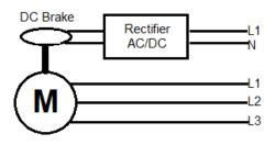
Figure 6. Example of DC brake motor connection.
