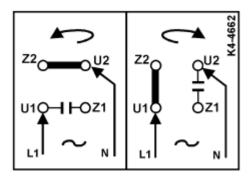
Figure 13. Single phase motor type SE(M)(K, L)h, with run capacitor.
