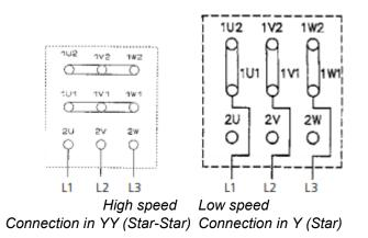
Figure 12. Three phase dual speed motor for ventilation application, with single windings (Dahlander), like 4/2-, 8/4-pole. 9 terminals. Motor marked with "W" on the motor data plate.
