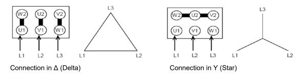
Figure 18. Standard three phase single speed motor.
