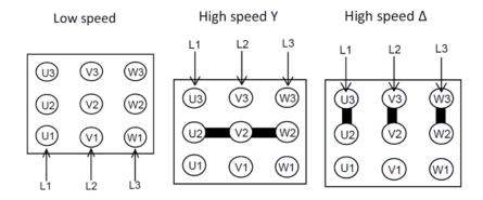
*Figure 20. Three phase dual speed motor with separate windings, like 4/6-pole. Y/D-start at high speed.*
