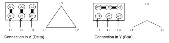
Figure 15. Standard three phase single speed motor.
