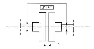
Figure 1. Using coupling on motor shaft.
