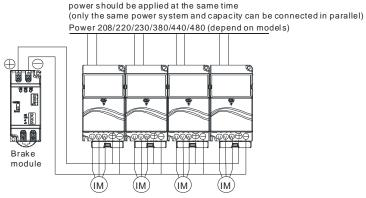
For frame A, terminal + (-) is connected to the terminal + (-) of the brake module. For frame B, C and D, terminal +/B1 (-) is connected to the terminal + (-) of the brake module.
