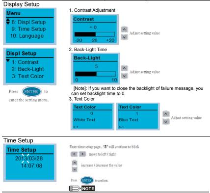
Limitations : The capacitor charging time of KPC-CC01 is around 6minutes. When the digital keypad is removed, the time setting will be in standby status for 7 days. After this period, the time needs to be reset.
