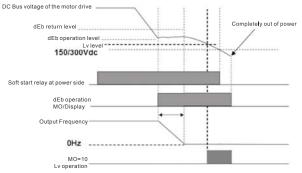
Exception: If the output frequency doesn't decrease to 0Hz yet and DC Bus voltage is lower than 150/300Vdc, the motor drive start to free run immediately and soft start relay is disconnected.
