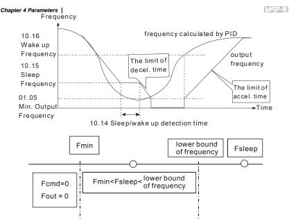
When Pr. 01.05min. output frequency ≤ PID frequency (H) ≤ Pr.01.08 lower bound of frequency and sleep function is enabled (output frequency (H) < Pr.10.15 sleep frequency and time > Pr.10.14 detection time), frequency will be 0 (in sleep mode). If sleep function is disabled, output frequency(H) = Pr.01.08 lower bound frequency.
