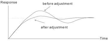
Example 3: How to suppress the oscillation of the wave with short cycle?
