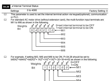
When extension card is installed, the number of the multi-function input terminals will increase according to the extension card. The maximum number of the multi-function input terminals is shown as follows.
