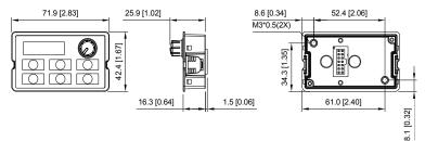
B.6.3 Digital Keypad Installation Method1. Install directly (Unit : mm [inch])
