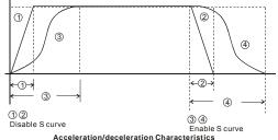
Related parameters: Pr.01.09(Accel Time 1), Pr.01.10(Decel Time 1), Pr.01.11(Accel Time 2) and Pr.01.12(Decel Time 2).
