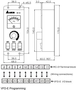
Pr.02.00 set to 2 Pr.02.01 set to 1 (external controls) Pr.04.04 set to 1 (setting Run/Stop and Fwd/Rev controls) Pr.04.07 (MI5) set to 5 (External reset) Pr.04.08 (MI6) set to 8 (JOG operation)
