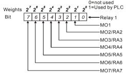
For example: when Pr.03.09 is set to 3 (decimal) = 00000011 (binary) that indicates Relay1 and MO1 are used by PLC. (Pr.03.09= $2^0+2^1=3$ )
