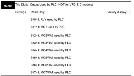
The equivalent 8-bit is used to display the status (used or not used) of each digital output. The value that Pr.03.09 displays is the result after converting 8-bit binary into decimal value.
