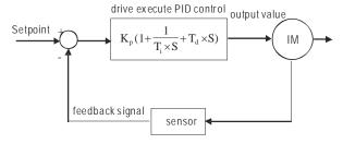
$K_p$ : Proportional gain(P)  $T_i$ : Integral time(I)  $T_d$ : Derivative control(D) S: Operator
